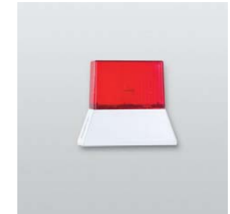
Visible warning device FSB flat strobe beacon Supply voltage 10.2 - 15 V DC ■ Calotte: Red ■ VdS class C (G 107055) ■ Type No. 100059711 Low supply voltage 16 - 30 V DC ■ Calotte: Red ■ VdS class C (G 107055) ■ Type No. 100059712 Supply voltage 230 V AC ■ Calotte: Red ■ Type No. 100059713
